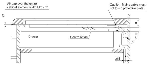
H Dimension from the top of the work surface to the underside of the hob (ventilation opening)
